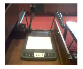
Document Cameras are available in each podium. The camera allows counsel to present evidence through video monitors. The evidence displayed can be of any medium including 3-D objects and x rays. The camera has many features; however, the ones you should be familiar with are highlighted below.
